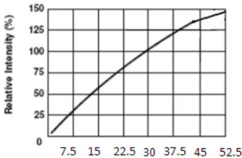
Fig 3. Relative Intensity Vs. Forward Current
