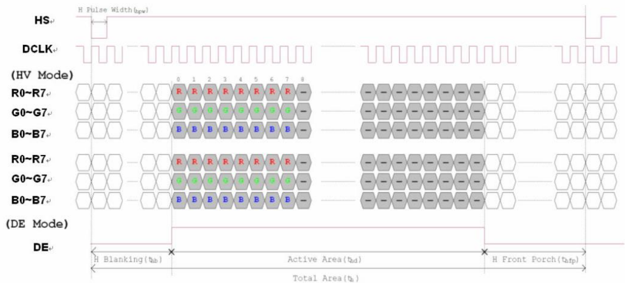
Horizontal input timing diagram.
